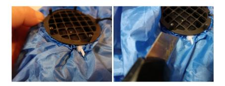
Locate & open the zipper. You should now be able to remove the old motor and old cord through the hole.
