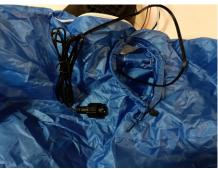
Fit the blower fan into the hole and tighten the ziptie to secure the blower fan in place.
